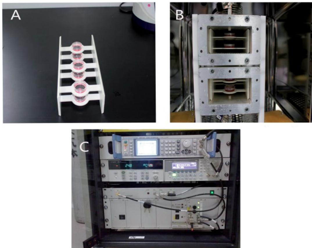
Figure 1. The sXc-1800-MHz exposure system. (A) Dish holder, (B) waveguides in an incubator, (C) signal generator.
